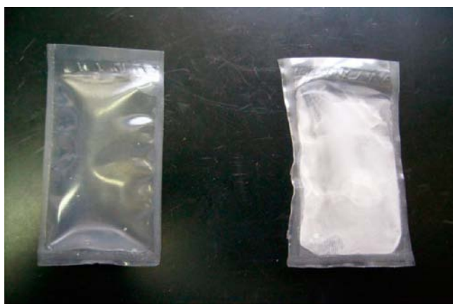
Figure 7. Images of LDPE packaging materials filled with Milli-Q water and exposed to -6 °C, one without any treatment (left) and the other UV-ozone-treated on the inner surface followed by LbL deposition to form \epsilon -PL/i-carr/ \epsilon -PL/ECIN multilayers (right).
