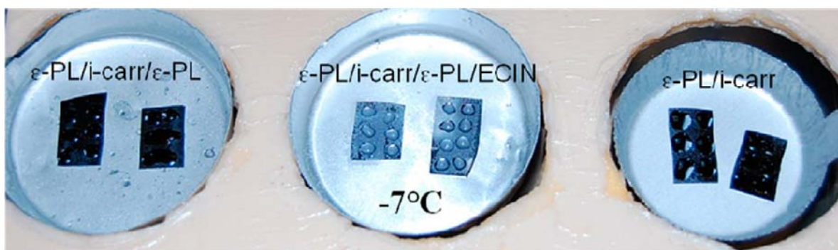
Figure 5. Freezing of 10 \mu\text{L} of high-purity dionized water droplets on ECIN, i-carr, and \epsilon -PL top layers at -7^\circ\text{C} .
